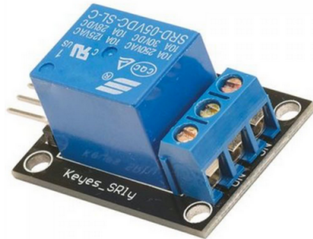
Figure 32: Example of Relay to be used
